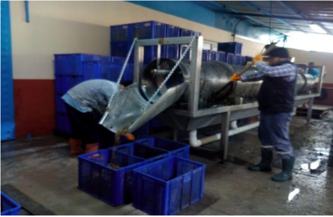
Figure 5. Washing of sea snails in the washing drum.
