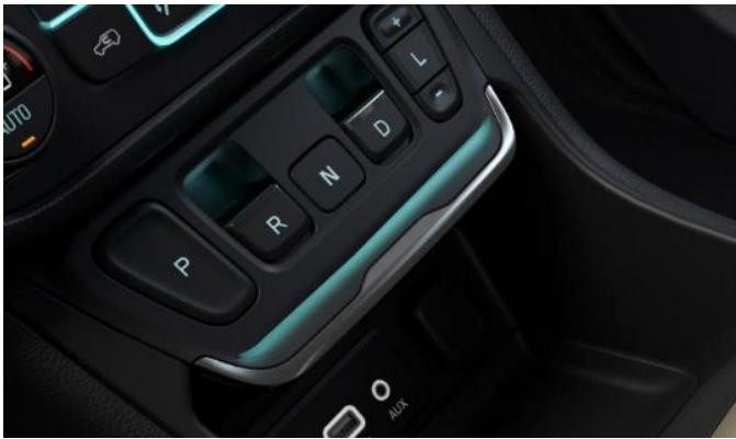
Figure 3. Shift-by-Wire System with button shifting (BestRide, 2016).
