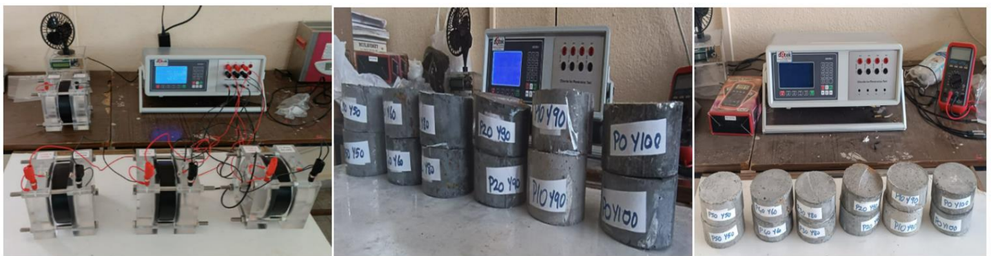
Figure 3. Chlorine permeability of AAS composite mortars.
