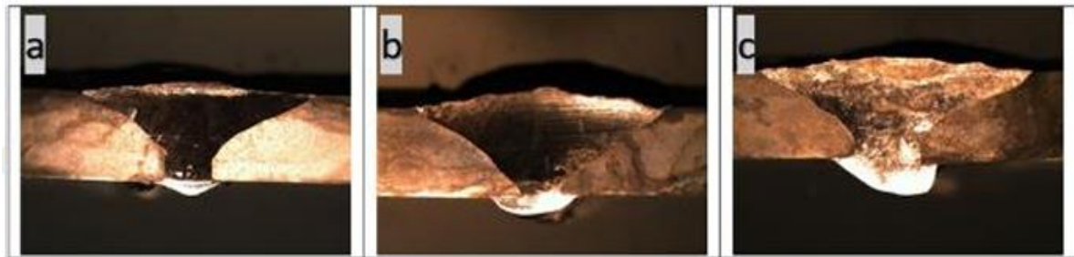
Figure 3. Macrostructure images of the welded joint made with the Citochromax coded electrode (Ø3.25 mm) a) N1, b) N2 and c) N3.
