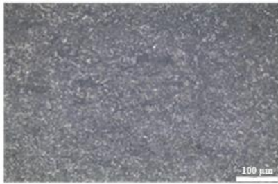
Figure 5. Microstructure images of Miilux Protection 500 base material.
