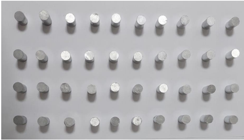
Figure 1. Macroscopic appearance of the Al–BFS composite samples produced with different BFS reinforcement contents.
